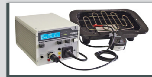
Testing an electric grill: PE | ISO | function
