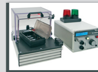
High-voltage test under a test cover
