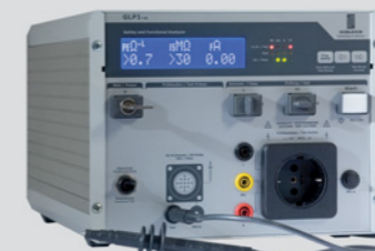
Testing device with up to 1500V DC
