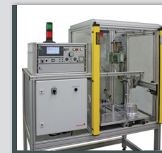
GLP2-e in a system solution with light curtain
