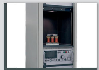
GLP2 in 19"-cabinet with high voltage 20KV AC
