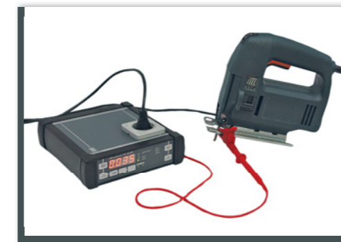
Testing PE and insulation resistance
