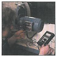
Performs complete fault detection of 3-phase squirrel-cage motors in a few minutes.
