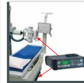
Testing the PE at X-ray equipment
