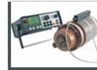
Winding detection at a rotor with induction test probe
