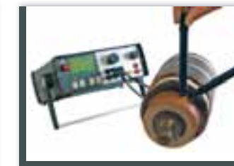
Resistance test at an armature between the lamellas
