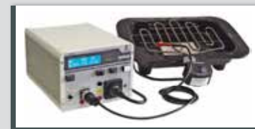
Testing an electric grill: PE | ISO | function
