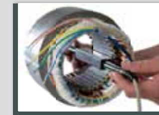
Winding detection at a stator with induction test probe
