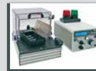
High-voltage test under a test cover
