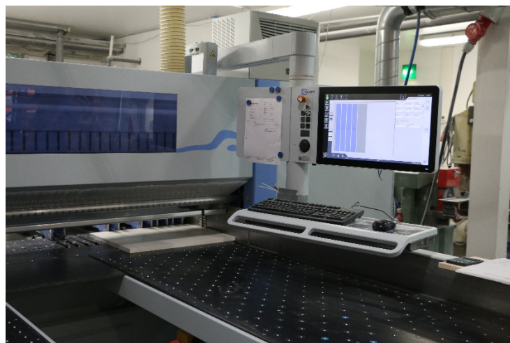
Automatic cutting of thicker sheet
