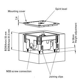
All standard socket outlets with an 80 mm cover and support ring fastening available for installation engineering, communication and telecommunications can be mounted into the 1632500 enclosure. To assist with installation, BOWAmini and BOWAmaxi include a mounting cover with spirit level as well as 4 height adjustment screws. Simple and safe connection with coupling brackets.
