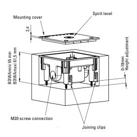
To assist with installation, BOWAmini and BOWAmaxi include a mounting cover with spirit level as well as 4 height adjustment screws. Simple and safe connection with coupling brackets.
