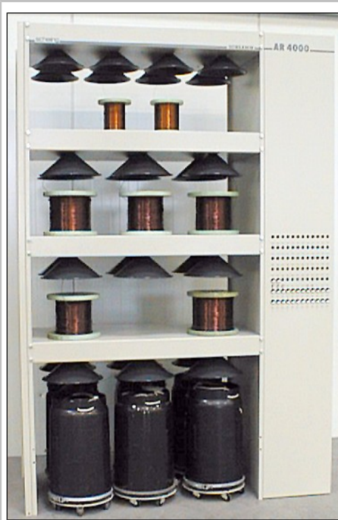
Picture: AR 4000 dereeling shelf with 90° panel, version for 8 x K200, 12 x K250, 6 long containers with wheel plates
