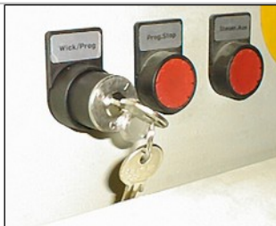
Picture: Key switch
